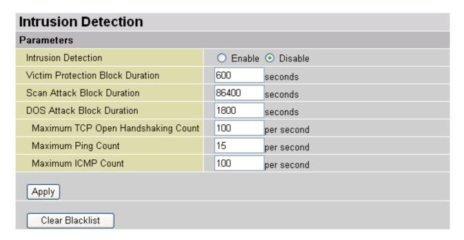
The router's *Intrusion Detection System* (IDS) is used to detect hacker attacks and intrusion attempts from the Internet. If the IDS function of the firewall is enabled, inbound packets are filtered and blocked depending on whether they are detected as possible hacker attacks, intrusion attempts or other connections that the router determines to be suspicious.
