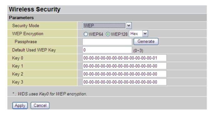
**WEP Encryption:** To prevent unauthorized wireless stations from accessing data transmitted over the network, the router offers highly secure data encryption, known as WEP. If you require high security for transmissions, there are two alternatives to select from: **WEP 64 and WEP 128.** WEP 128 will offer increased security over WEP 64.
