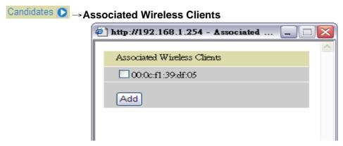
Associate Wireless Client displays a list of individual wireless device's MAC Address that currently connects to the router.
