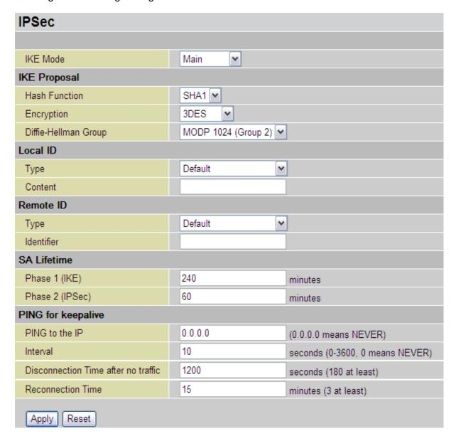
**IKE (Internet key Exchange) Mode:** Select IKE mode to Main mode or Aggressive mode. This IKE provides secured key generation and key management.
