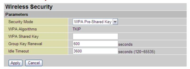
**WPA Algorithms:** TKIP (Temporal Key Integrity Protocol) utilizes a stronger encryption method and incorporates Message Integrity Code (MIC) to provide protection against hackers.
