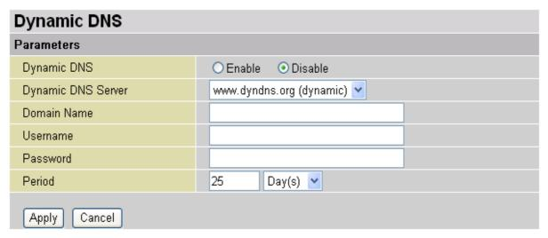
The Dynamic DNS function allows you to alias a dynamic IP address to a static hostname, allowing users whose ISP does not assign them a static IP address to use a domain name. This is especially useful for hosting servers via your ADSL connection, so that anyone wishing to connect to you may use your domain name, rather than having to use your dynamic IP address, which changes from time to time. This dynamic IP address is the WAN IP address of the router, which is assigned to you by your ISP.
